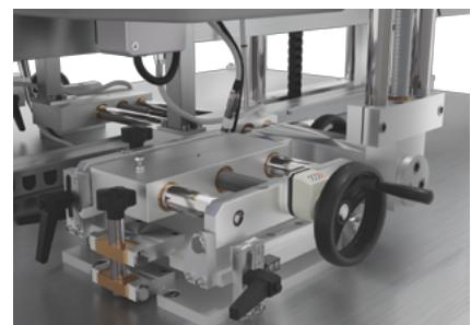
*Labelling head support with micrometric adjustment.*
